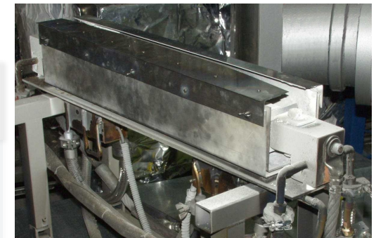
Metal sublimation equipment designed by FEP & tested in MAXI
