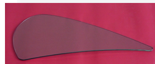
PC window of a passenger car, both side coated with \text{SiO}_x
