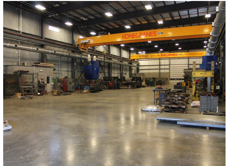
Weld Shop, 2 25ton Cranes
