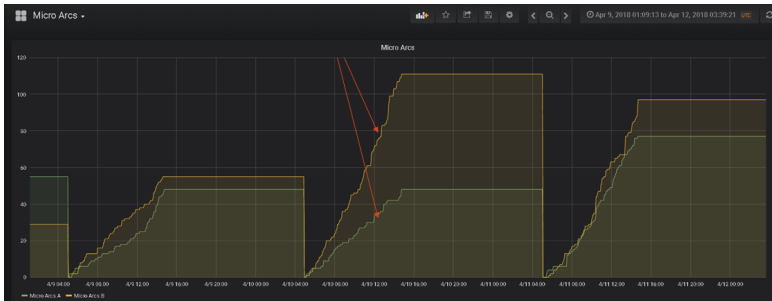
Case 1 Arc rate is substantially higher on one cathode versus other during operation – indicates potential issue
