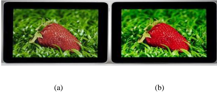
Figure 9. LCD displays without (a) and with (b) 3M QDEF.
