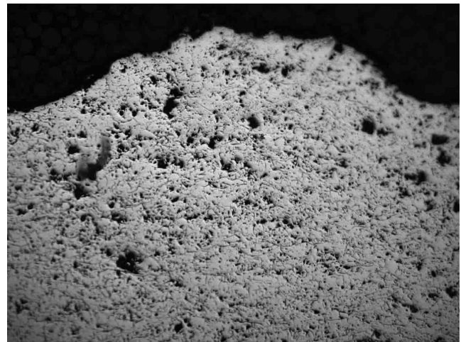
Figure 3: Optical micro-graph from a cross section through a nodule on a sprayed silicon target.
