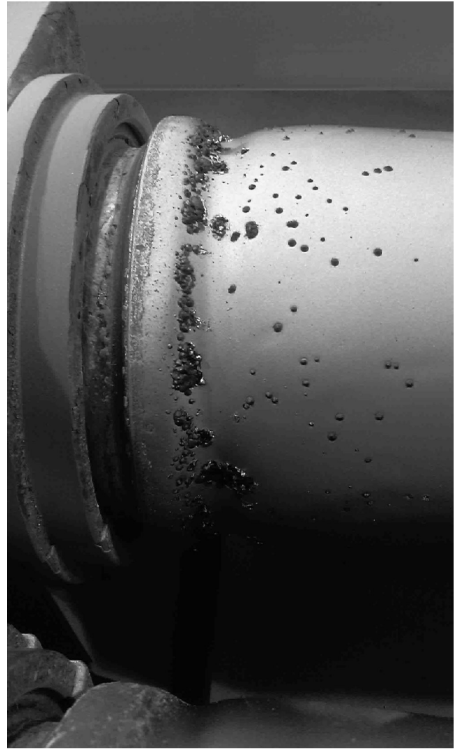
Figure 2: Nodules generated on a sprayed Si target used in a reactive process to sputter SiO 2 -coatings.
