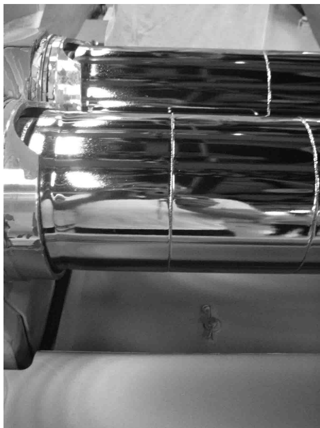
Figure 9: Detail of a few of the gaps between cast-Si cylinders after 25,000 kWh of accumulated energy load on the set.
