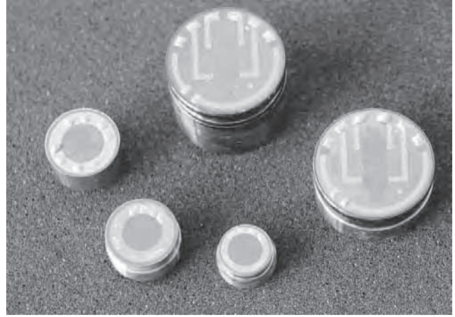
Figure 3: Pressure sensors based on metal membranes with sputtered insulating layers and structured resistive and contact layers (Sievert TFT).
