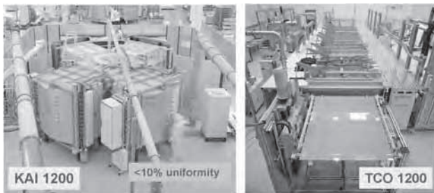
Figure 3: On the left, a PECVD KAI 1200 system, on the right a TCO 1200 system for fabricating a-Si modules on 1.4 m 2 [13].
