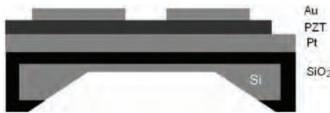
Figure 2: Schematic of pMUT layers.
