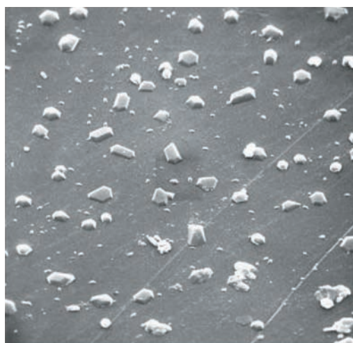
Figure 8: A micrograph of Melinex '442' that has been subjected to prolonged heating at 140°C. Scanning electron microscope Magnification 2000x. Showing the growth of 'mer' (dimers, trimers..... hexamer) units into substantial crystals.
