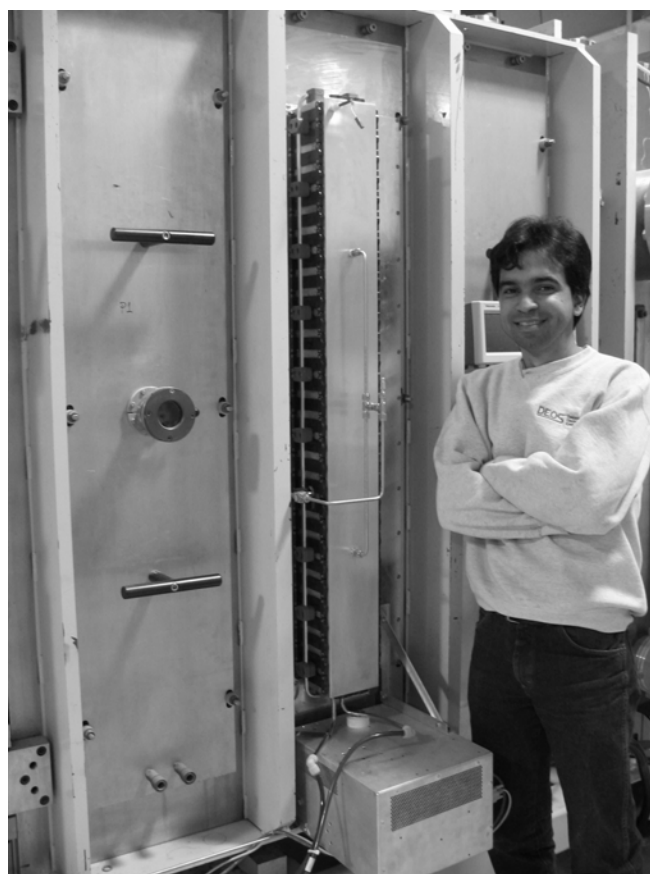
Figure 3. Rectangular source mounted on the test station. Source length is 1.3\text{ meters} , with an interior cross-section of 10\text{ cm} \times 10\text{ cm} .
