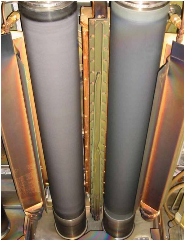
Figure 1. Two rotatable ITO targets mounted in a production scale in-line sputtering chamber.
