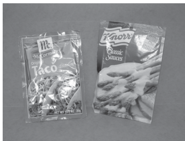
Figure 4: Samples of Paper-Poly-Foil-Poly Pouches. Wrinkles on the pouches were present when taken from shelf.
