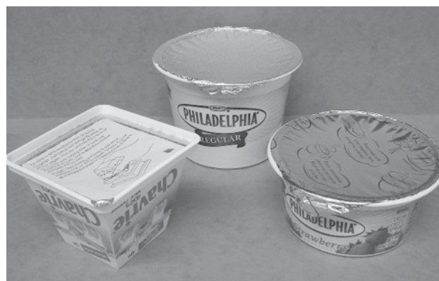
Figure 3: Samples of cheese in PP Cups: Lids of the two left samples are made from 60 – 65 mm aluminum foil. The right lid is a Poly-Foil-Poly laminate with a total thickness of ~80 mm. This type of lid typically shows better printing.
