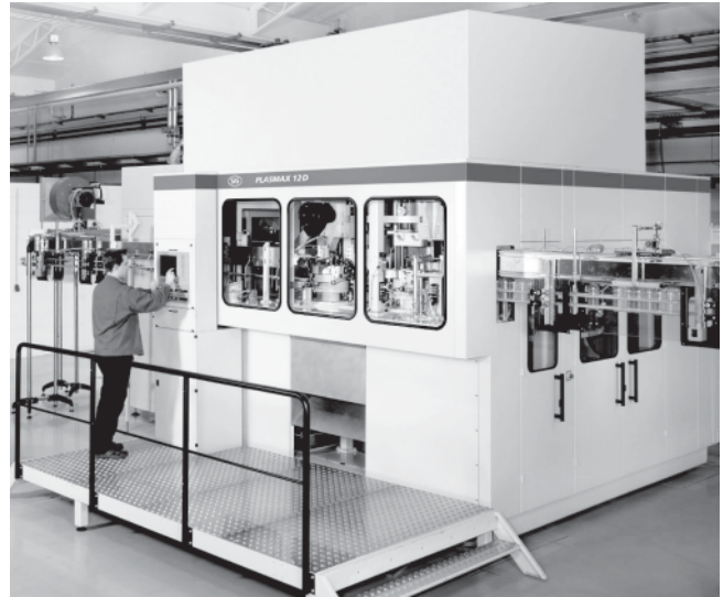
Figure 4: PCVD bottle coater with 12 double stations based on a SBM (courtesy of SIG).
