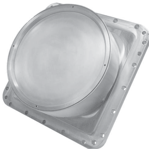
Figure 2: Planar magnetron for 8" circular targets and with complete freedom for positioning magnets
