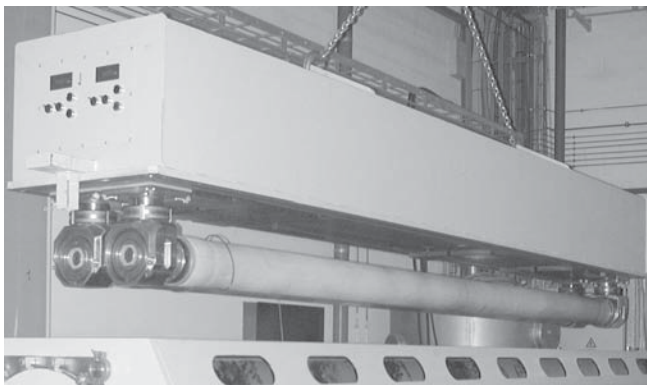
Figure 3: Experimental set-up for large area uniformity testing containing a dual rotatable magnetron
