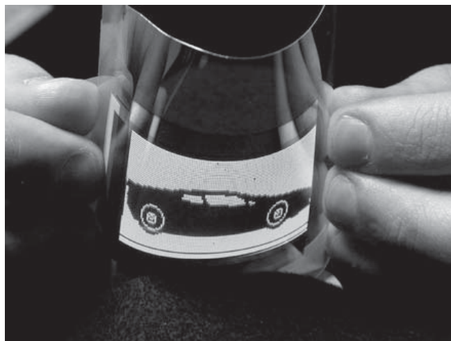
Figure 1: A 128 x 64 FOLED passive matrix display fabricated on a 0.175 mm polyethylene terephthalate substrate (PET) shown being driven at a video rate of 60 Hz and an average display brightness of 200 cd/m 2 . Each pixel is 400 x 500 \mu m in size.
