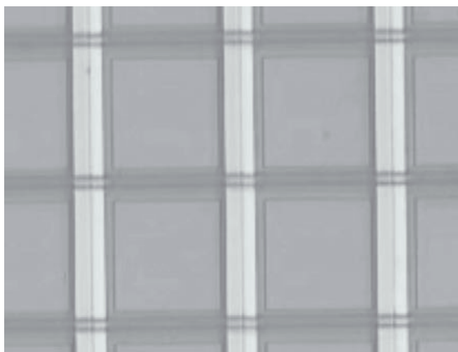
Figure 5: This is a magnified view of a patterned flexible substrate. The pixel pitch is for an 80 dpi resolution display. The active pixel area is defined by each square.
