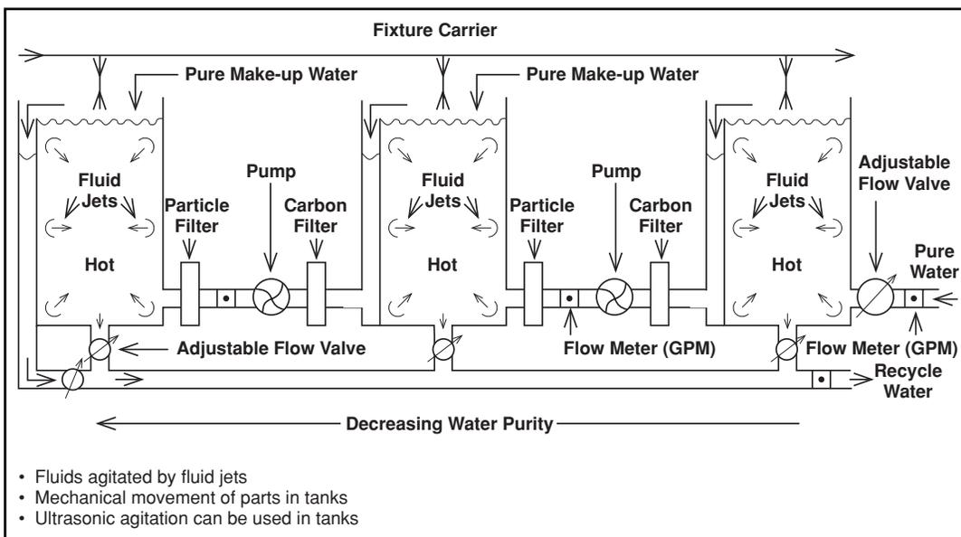
Figure 1: A cascade rinse system gives a very high level of cleanliness to the final rinse.
