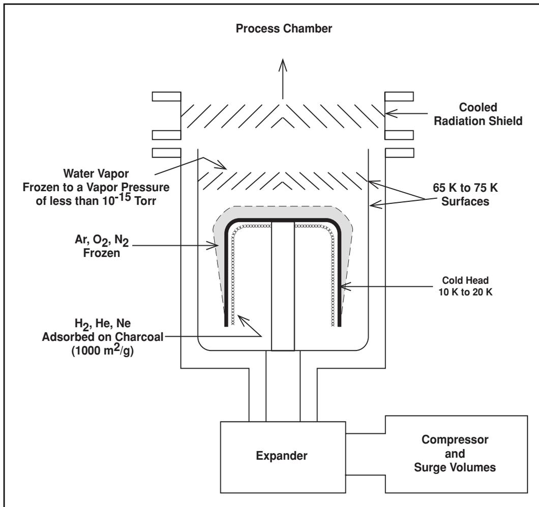
Figure 1: Cryopump with radiation shield.
